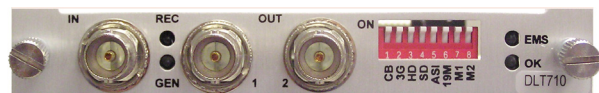
Rear panel includes electrical video and audio signal generator and checker, and format select switches
